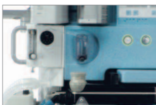
Integrated Oxygen Therapy featuring O 2 supply up to 12 L/min and mechanical airway pressure monitoring.
